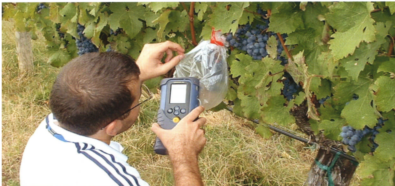
In the field, a handheld electronic nose measures grape maturity. A bag surrounds a cluster and contains the volatiles.
