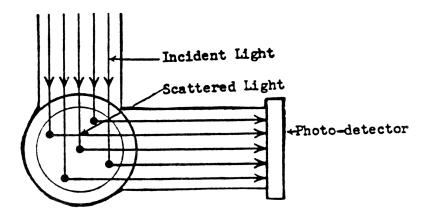
Figure 1 Schematic Representation of a Nephelometric Measurement
